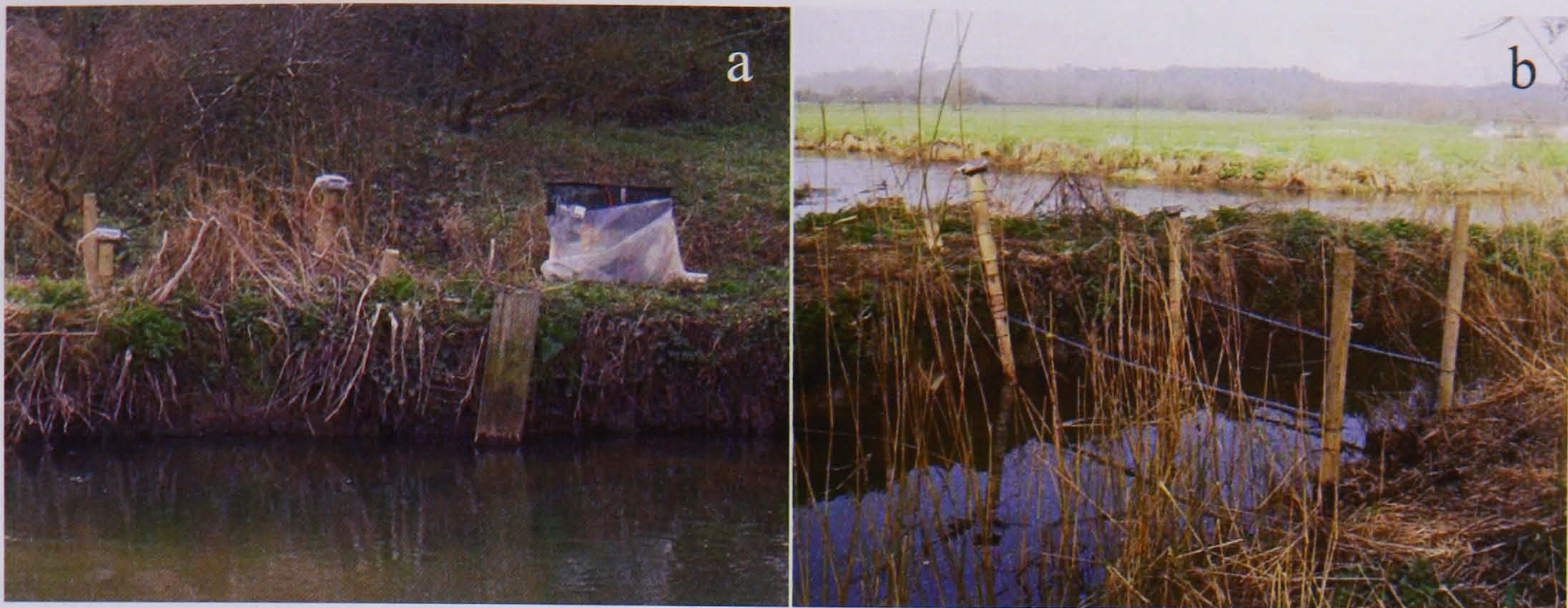
Figure 3.7 TIRIS PIT detector at Luckford Lake showing (a) the protective box holding batteries and detector electronics on the bank (the stream channel runs parallel behind the main river channel in view) and (b) the two antenna.
