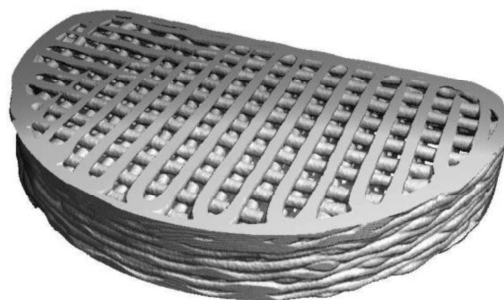
Figure 1. \mu\text{CT} 40 scan of a fabricated scaffold
