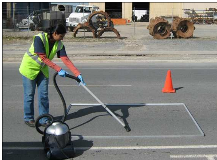
Figure 4.7: Collection of build-up sample through dry vacuuming
