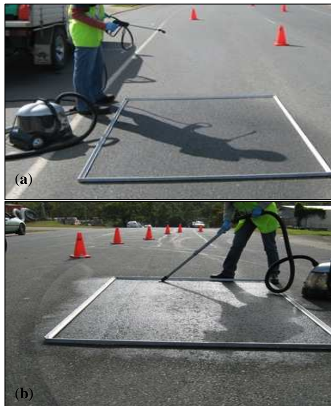
Figure 4.8: Collection of build-up sample through wet vacuuming: (a) Spraying and (b) Wet sample vacuuming
