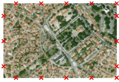
(a) Planar Landmark Selection: Border. The 16 landmarks are spaced at regular intervals around the map border.
