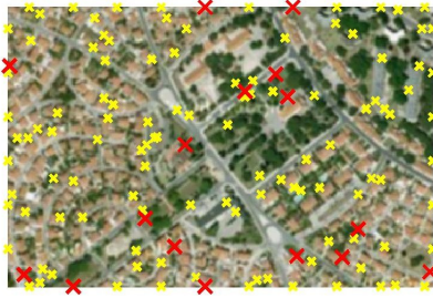
(d) Simple K-Medoids. Yellow crosses denote members of the candidate set of landmarks passed to the K-Medoids function, the candidate set contains both landmarks spaced around the border of the map and a large number randomly scattered in the internal section of the map.
