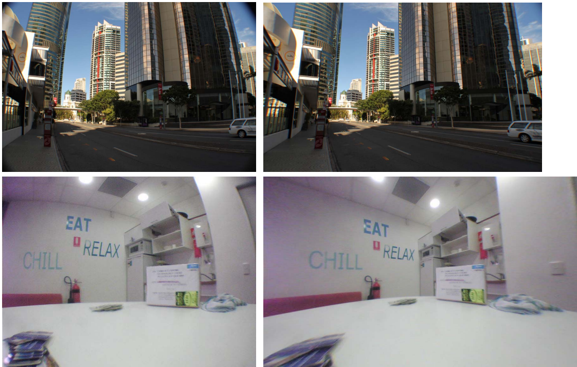
Fig. 5. Images distorted by real wide angle camera lenses (left) and automatically undistorted images (right).
