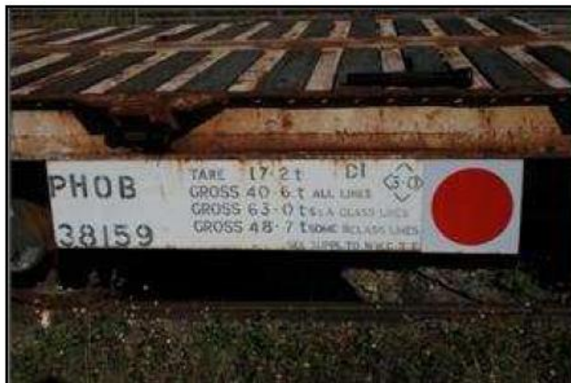
Figure 5.3 PHOB type wagon with identification plate (PHOB 38159) containing wagon type and information on the load carrying capacity
