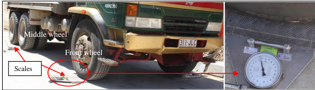
Figure 6.2 Measurement of wheel load at site
