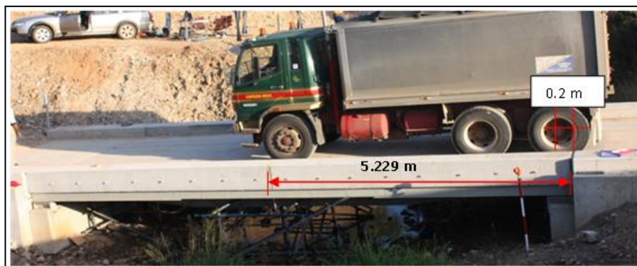
(b) Wheel locations for maximum shear
