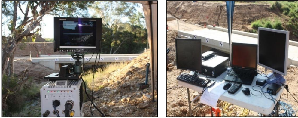
Figure 6.15 High-speed camera and computers set-up at site
