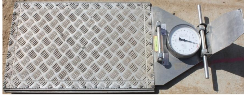
Figure 6.1 Portable weighing scale used to measure the wheel load
