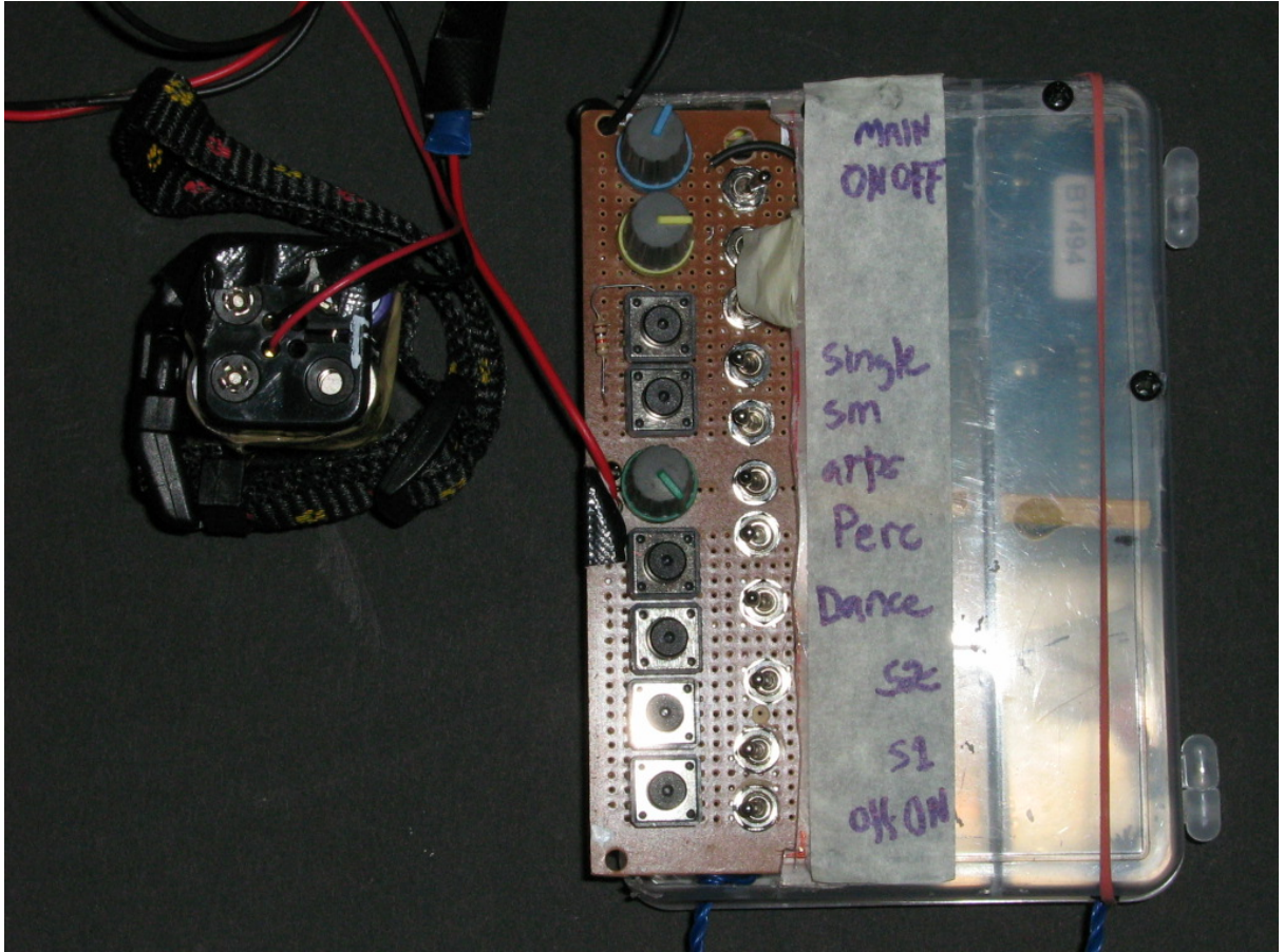
Figure 44. The Arduino controller, with battery pack worn in the performer's pocket. The written functions are for the toggle switches, whilst the push buttons and knobs have functions determined by the layer of the menu display.
