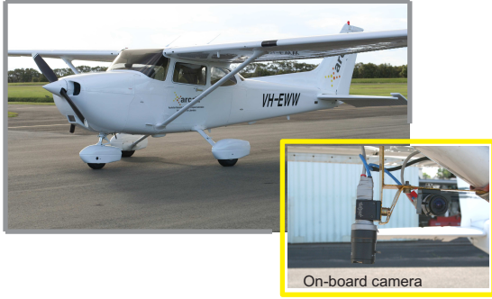
Fig. 3. Airborne System Laboratory (ASL). This laboratory consists of a Cessna 172 equipped with an x86 computer running Linux; a NovAtel SPAN, which computes a tightly-coupled GPS/INS solution for position and attitude data; two cameras: one pointing forwards and the other one pointing downwards; and custom electronics for data synchronization. The ASL is capable of capturing images at a rate of 30 HZ with a resolution of 1024 \times 768 .
