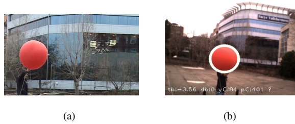
Figure 7: Object Following test using a fuzzy controller on a Pelican quadrotor:(a) External view of the tests using a colored balloon. The balloon is manually moved with a random trajectory, (b). The onboard image captured, and the projected diameter on the image plane identified using the Camshift color tracked.
