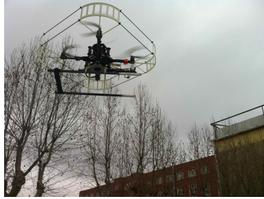
Figure 5: CVG-UPM [22] Pelican QuadCopter testbed used for sense and avoid experiments
