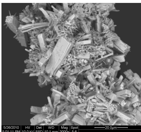
Fig. 6.3c – SEM micrograph of synthetic trippkeite
