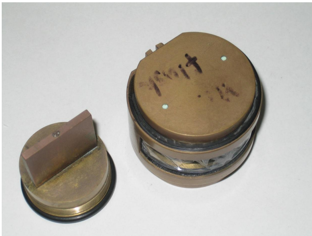
Figure 4.1: Inert atmosphere XRD stage
