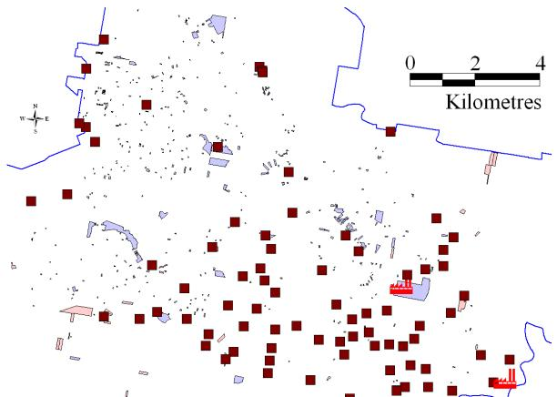
Figure 1. GIS Map of Springwood to Eagleby - an excerpt of the complaint locations (blue and red shaded properties) versus pumps (maroon squares) and treatment plants (red icons)
