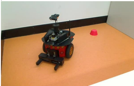
Fig. 2. The robot in the experimental 3x3m walled environment. The red, and other (green) markers, can be detected using the gripper while the wall and floor cannot.
