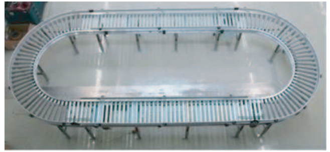
Fig. 6. Components of the conveyor line mechatronic system. The components are the straight segments, curved segments and drive mechanism.
