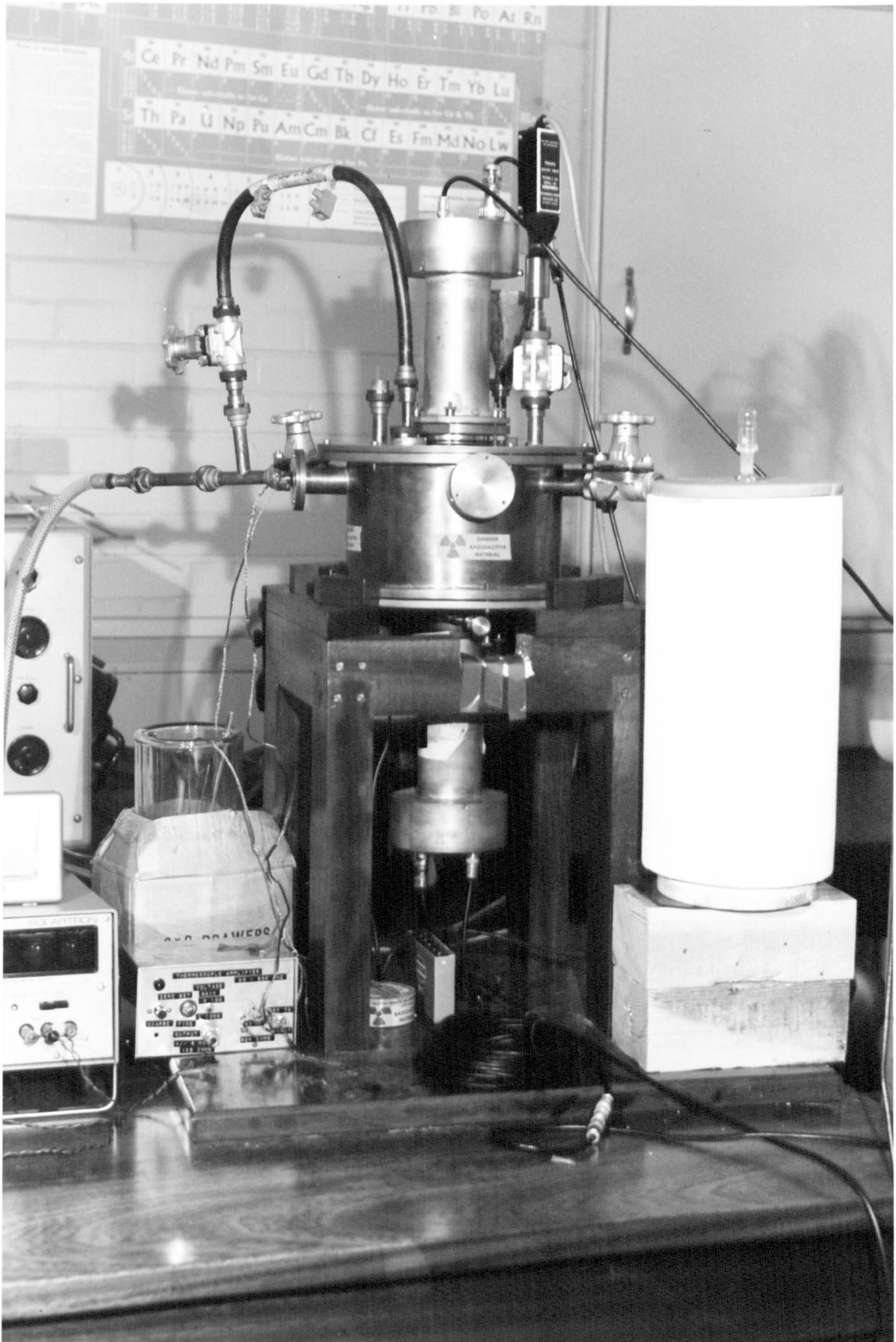
FIGURE 4.4 A general view of the decay system cryostat used with single-photon counting technique
