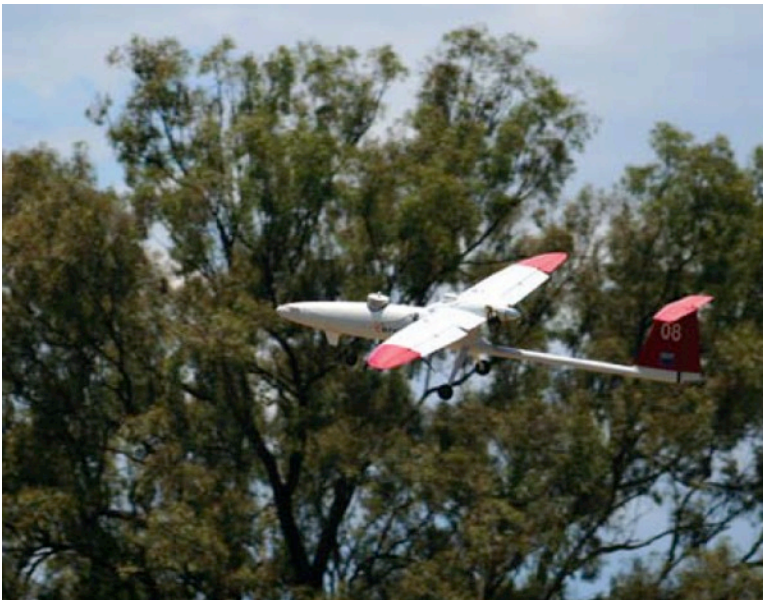
ARCAA UAS with plant disease-spore detection sensor fitted
