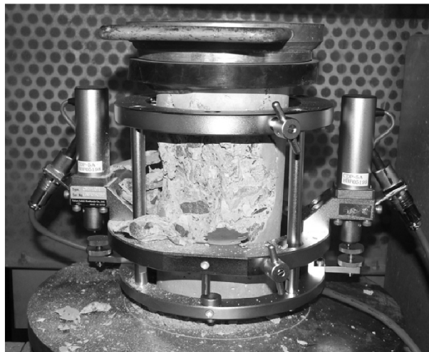
Figure 3.6: Concrete Compression Test Cylinder.
