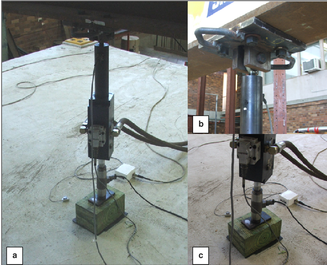
Figure 3.5: Hydraulic Ram and Load Cell – a) assembly; b) ram fixing to header beam; c) load cell mounted to ram and contact with floor on steel plate and timber block.
