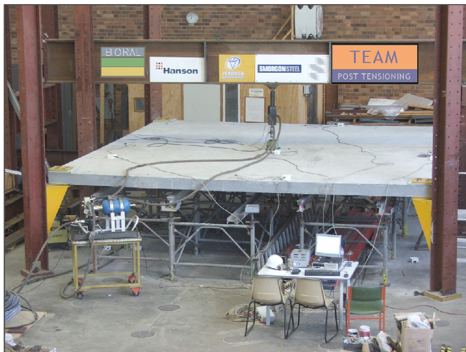
Figure 3.3: : Specimen Test Set-up: Hydraulic pump and actuator (bottom left); Data acquisition system (bottom right); Hydraulic ram/load cell fixed to header beam (top)
