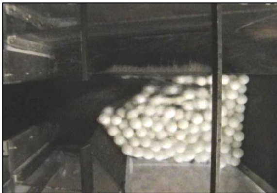
Figure 9. Deposition pattern for the GPT with 68% blocked screen shows total (100%) capture/retention of the lightest pollutants ( RD = 0.1) at a high (35 L/s—Table 1) flow rate (See C, Figure 10).
