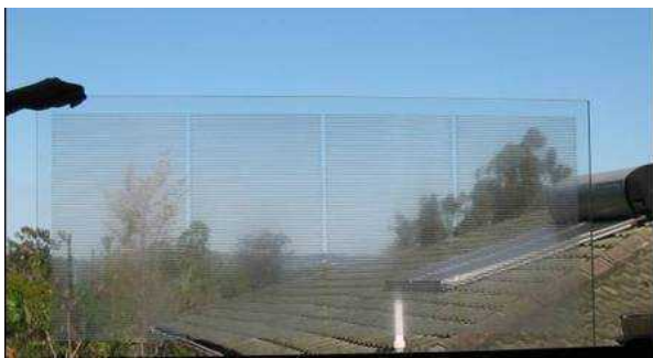
Figure 5: A laser cut panel (LCP) [10].
