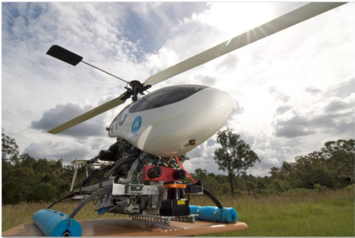
Figure 4 – The ARCAA autonomous unmanned helicopter with integrated SSA payload
