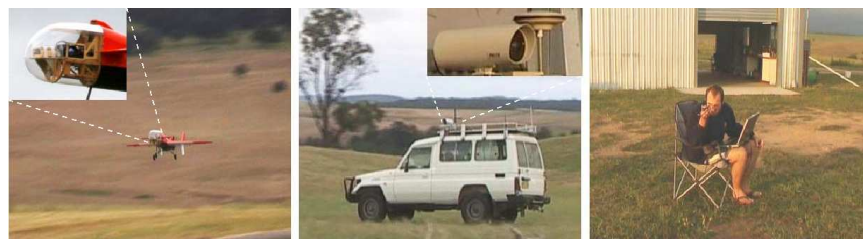
Fig. 4. Data is obtained from multiple sources including cameras mounted on an autonomous air vehicle and ground vehicle. Observations are also submitted to the system by human operators. Each of the different sensor modalities are incorporated into our filtering scheme. Close-ups of the sensor payloads including monocular colour cameras are shown in the insets.
