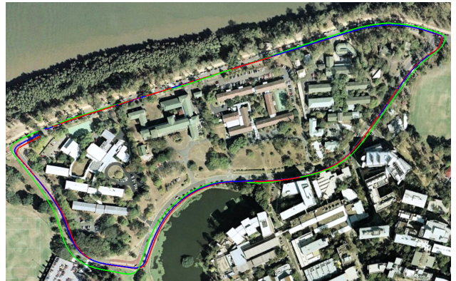
Figure 1: Comparison of unaided visual pose estimates (non-bundle adjusted trajectory in red, bundle adjusted trajectory in blue) with GPS (green) on data gathered by the platform overlaid on a satellite image.
