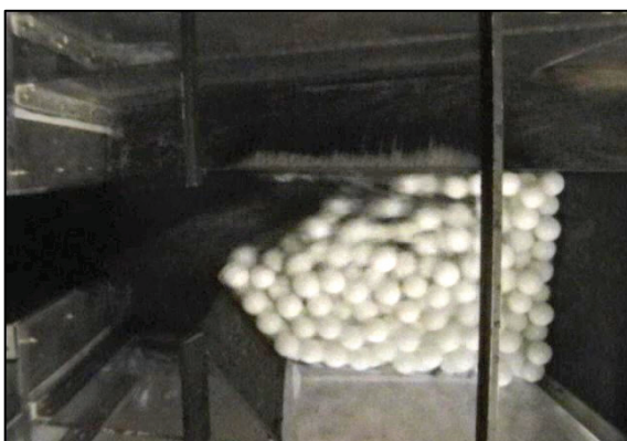
Figure 9.9 Deposition pattern for the GPT with 68% blocked screen shows total (100%) capture/ retention of the lightest pollutants (RD = 0.1) at a high (35 L/s) flow rate (See C, Figure 9.10).
