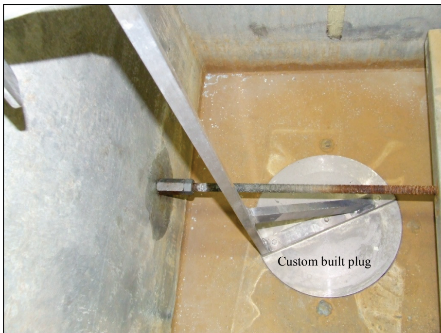
Figure D.3 The custom built plug used in the collection tank to measure the flow rate. The flow rate was calculated by timing the amount of water collected at a marked height in the tank.
