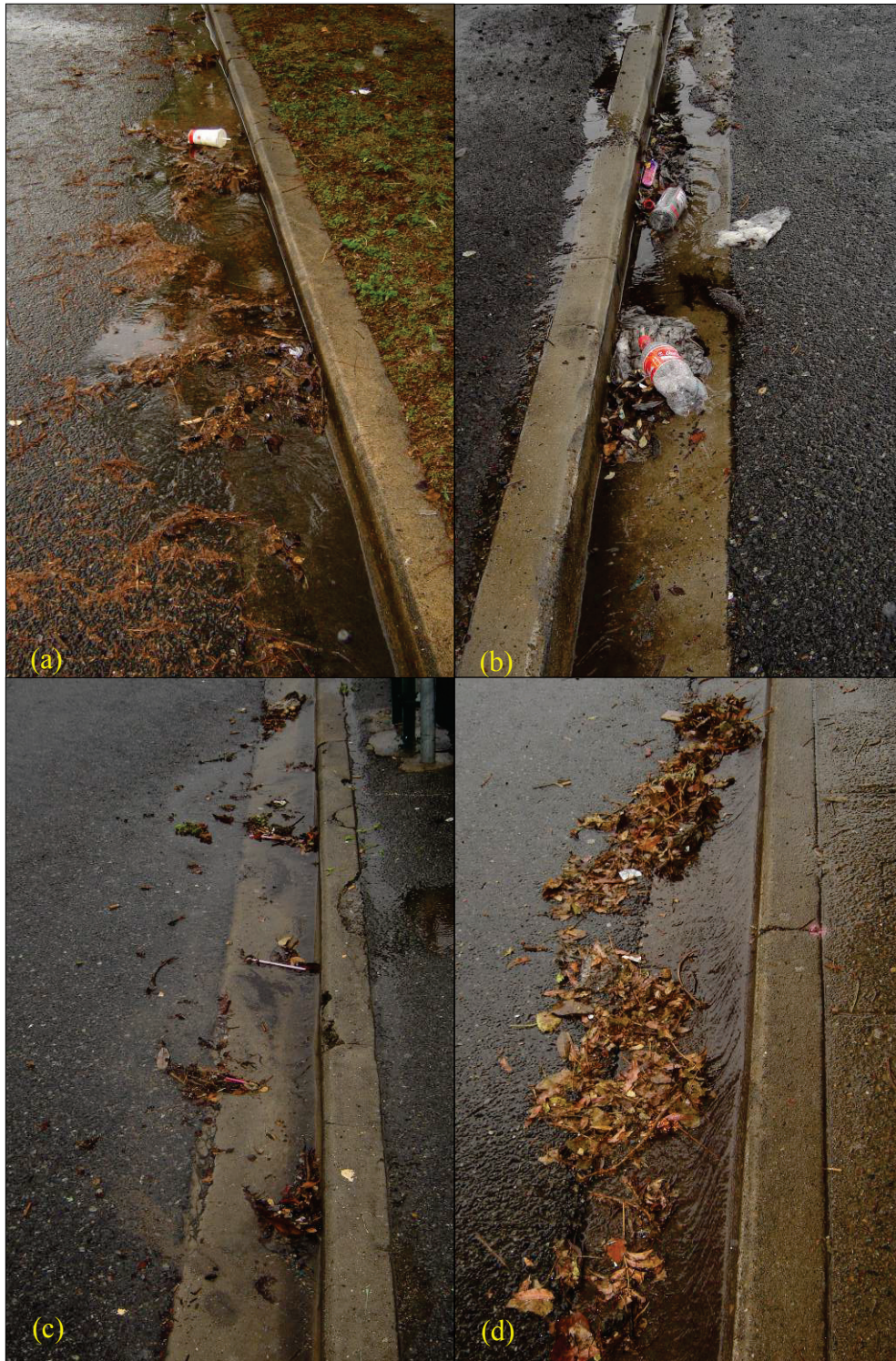
Figure 4.28 Flow characteristics of various organics during light rainfall: (a) accumulation of smaller matter into a mulch formation; (b) mainly litter with some organics; (c) twigs and small litter items and (d) leaves and twigs.
