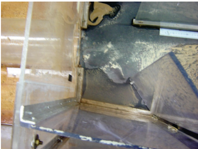
Figure F.27 A view of the area behind the baffle and the top left corner of the bypass channel in the GPT.
