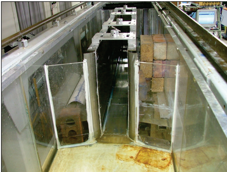
Figure D.7 Upstream view of the rectangular channel inlet GPT.
