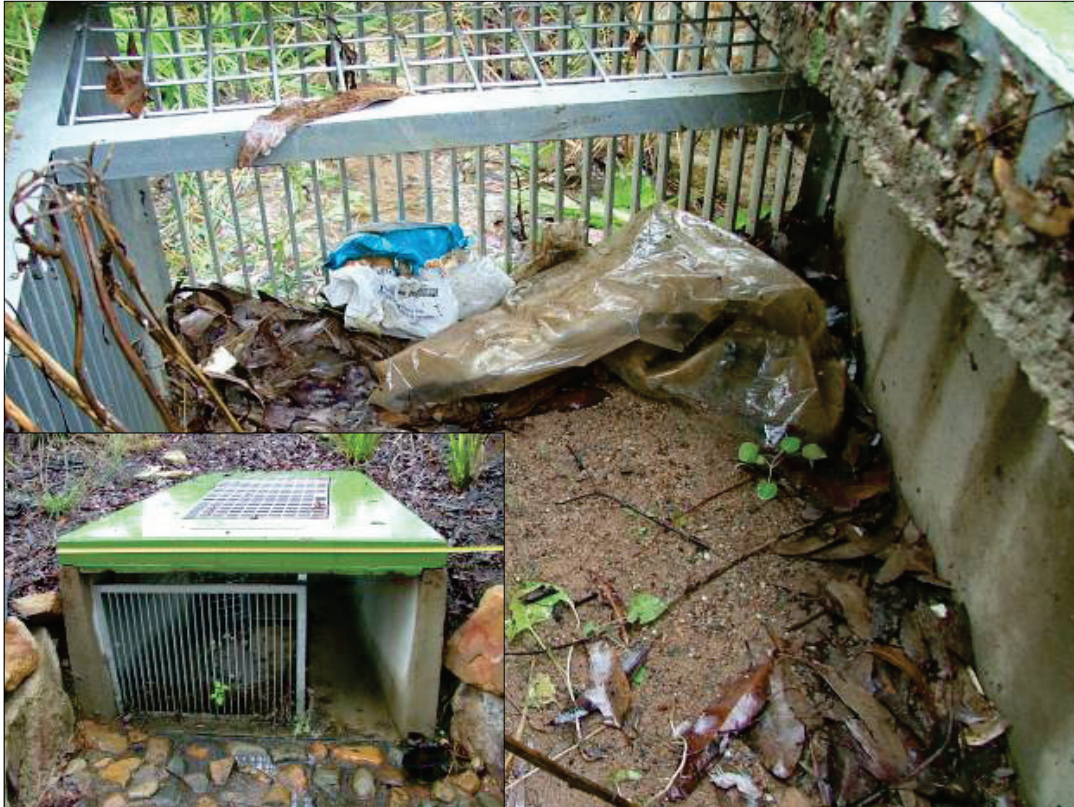
Figure 4.23 Field monitoring of the LitterBank GPT at a residential catchment area in an outer suburb of Brisbane (Marsden Park). The surrounding area is similar to the view shown in map of Figure 4.22. The capture of mainly fine sediments was due to a nearby construction site of new houses.
