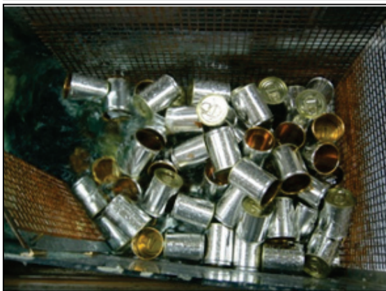
Figure 9.5 Left, A snapshot of a fully blocked GPT taken from litter deposit experiments with tin cans. The partially blocked GPT is modelled with all five polystyrene blocks (see blocks 1-5, Figure 9.3).
