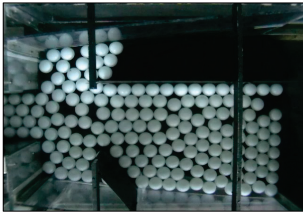
Figure 9.11 Single layer deposition pattern for the GPT with 68% blocked screen capture/retention of the lightest pollutants ( RD = 0.9) at a low (3.9 L/s) flow rate (See D, Figure 9.10).
