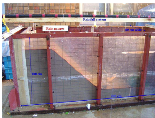
Figure 5. Tank used for model test
