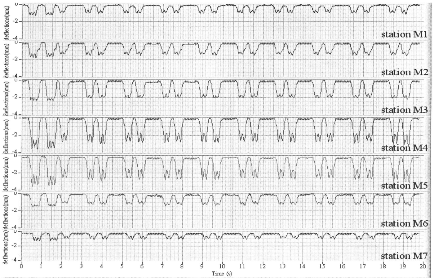
Figs. 5.1 to 5.7 showing the vertical deflection of the sleepers with the passing of 12 cars
