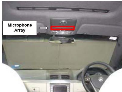
Figure 1: Position of microphone array inside car cabin.
