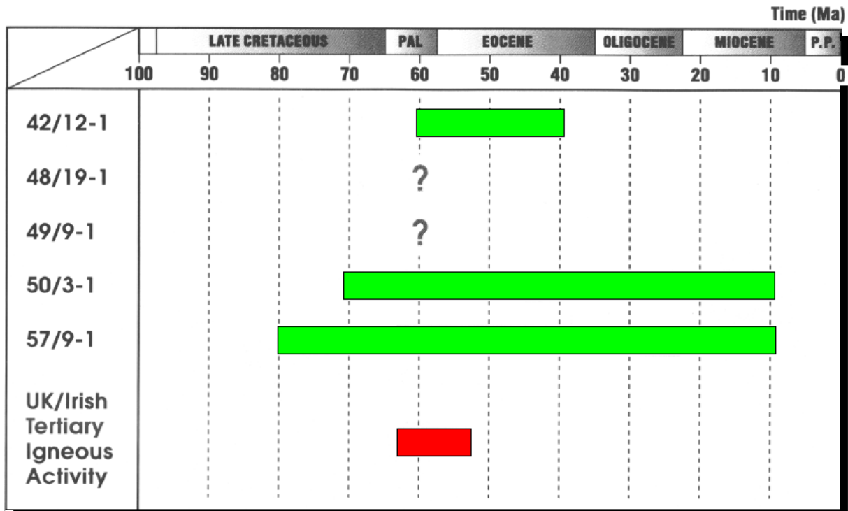
Figure 6.9 – Graph showing time of cooling from maximum palaeotemperature (from AFTA) for five wells compared to the timing of the Cenozoic igneous activity. Results are consistent with a widespread early Cenozoic uplift at around 60-55Ma, the time of the UK/Irish Cenozoic igneous activity. For two of the NCSB wells, results are also consistent with a later episode of uplift at 20Ma (modified after Murdoch et al. 1995).
