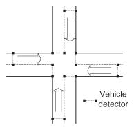
Fig. 2. Junction setup with vehicle detectors.
