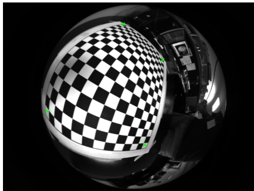
(a) Initial image with 4 corner points selected manually.
