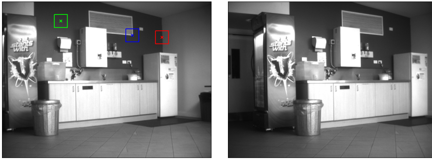
(a) Two images separated by a change in viewpoint. Image 1 (left) shows a corner point (blue), edge point (red) and homogeneous point (green). The square region surrounding each is used for the cross-correlation
