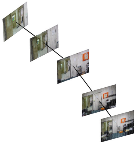
(c) Estimated relative camera pose of each image in the sequence obtained using a structure from motion algorithm.
