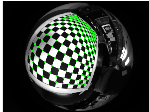
(d) Position of grid points mapped back to the original image. This is the input data used for full calibration.
