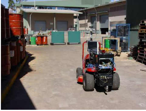
Fig. 7. CSIRO Autonomous Tractor in a canyon with an L-junction at the end
