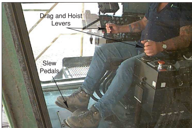
Figure 3. Operator controls. Two hand levers control the drag and hoist axes whilst a pair of foot pedals control the dragline slew motion.
