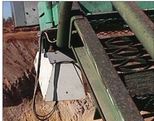
Figure 10. The laser scanner mount at the dragline's boom tip.
