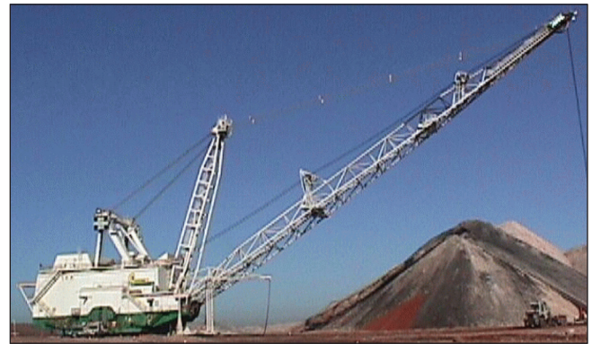
Figure 1. A Bucyrus-Erie 1350 dragline. For scale, note the large truck in the lower right corner of the photograph. Typical boom lengths are 100 m.
