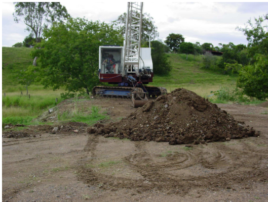
Figure 8: Photo of spoil pile after 50 autonomous cycles with the scale dragline in the background.
