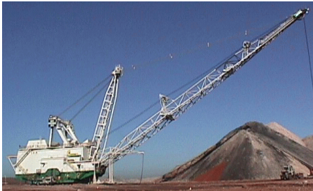
(c) 3500 tonne dragline.
