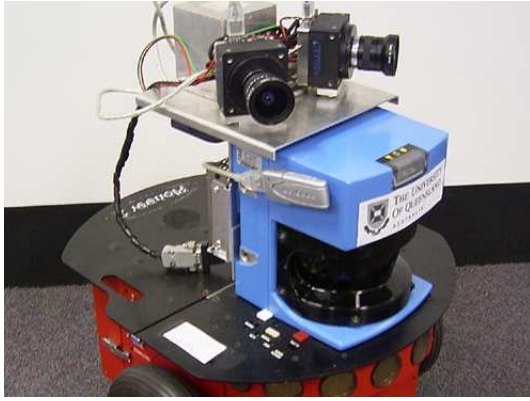
Figure 1: The Pioneer robot including a SICK laser, sonar ring, two Basler cameras and the EiMU sensor.
