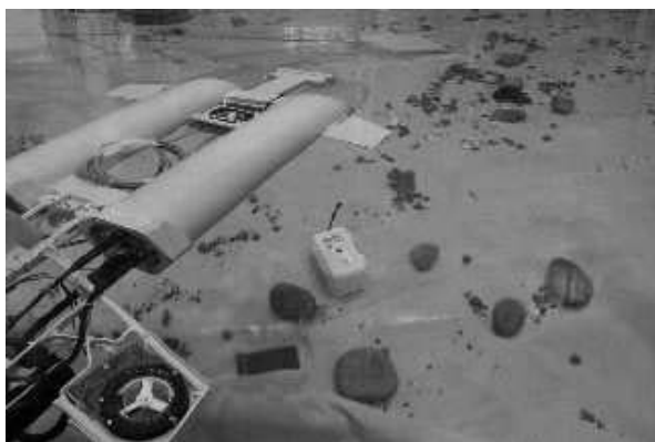
Figure 2. A small AUV interacting with the underwater Flecks in a “simulated ocean”.
