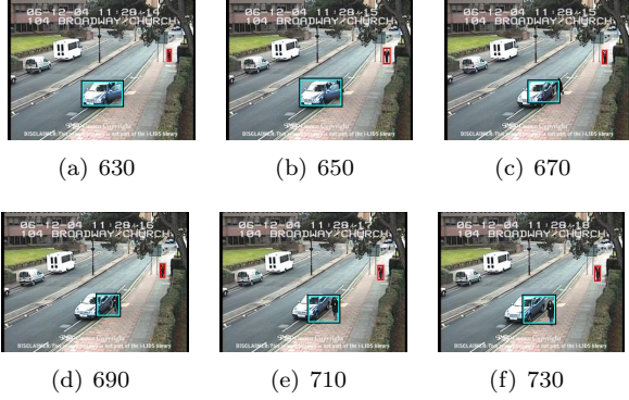
Figure 4. Sample Tracking Output - Errors tracking a stopped vehicle.
