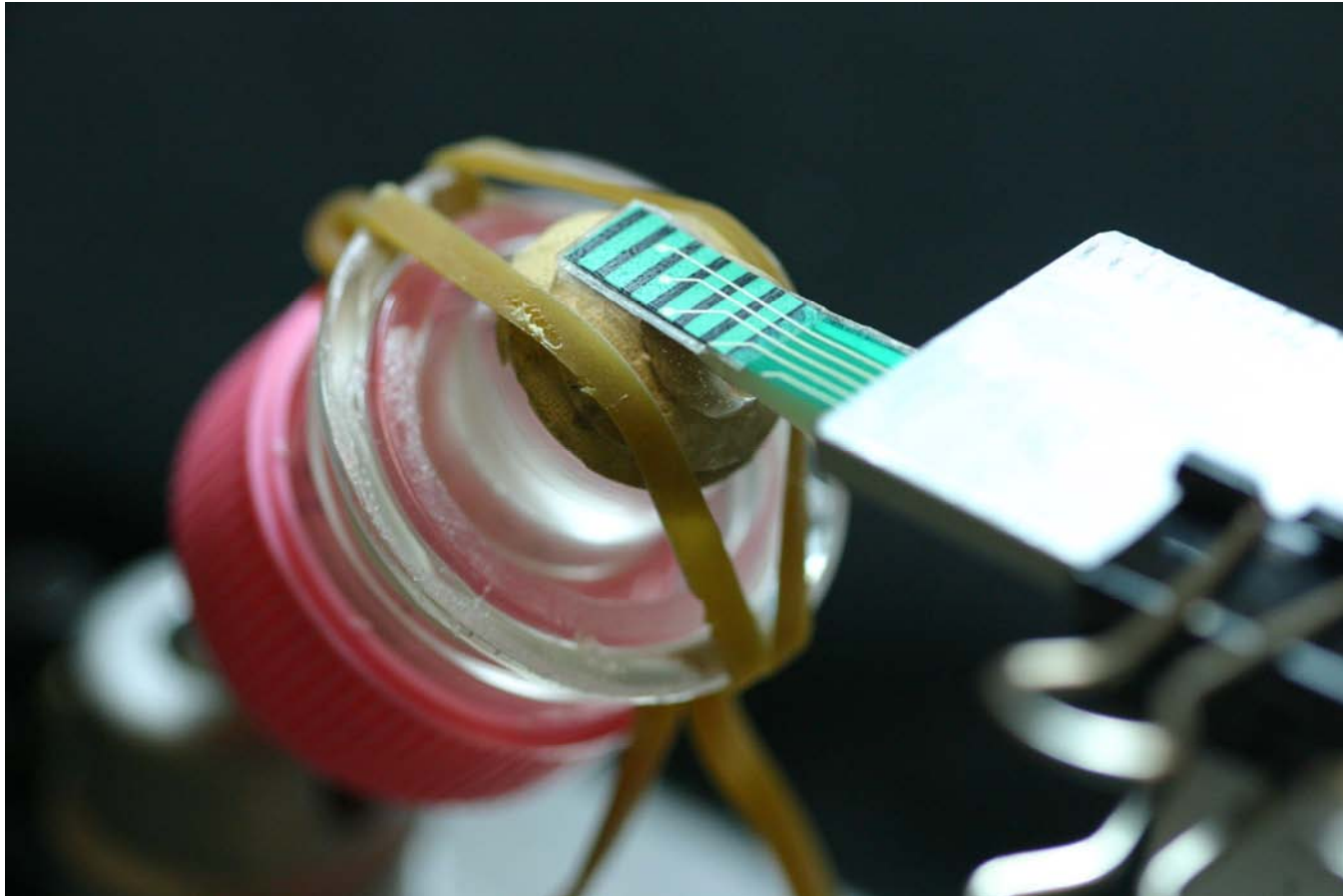
Figure 3-8: The sensor-contact lens combination in the rubber band holder simulating eyelids on the lens. There was no output change with the rubber bands so it can be assumed that there was no flexure of the contact lens surface over the region to which the sensor was attached.
