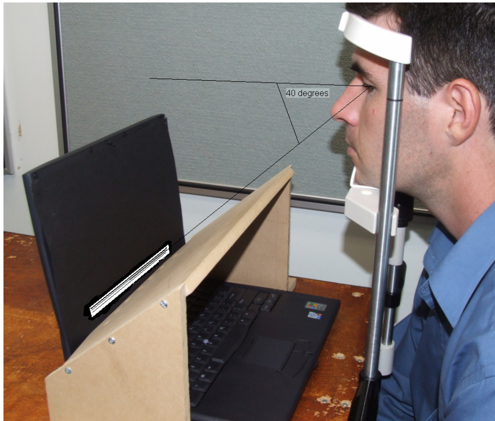
Figure 2-2: Visual task positioned at 40° downward gaze, approximately 40 cm from the subject.
