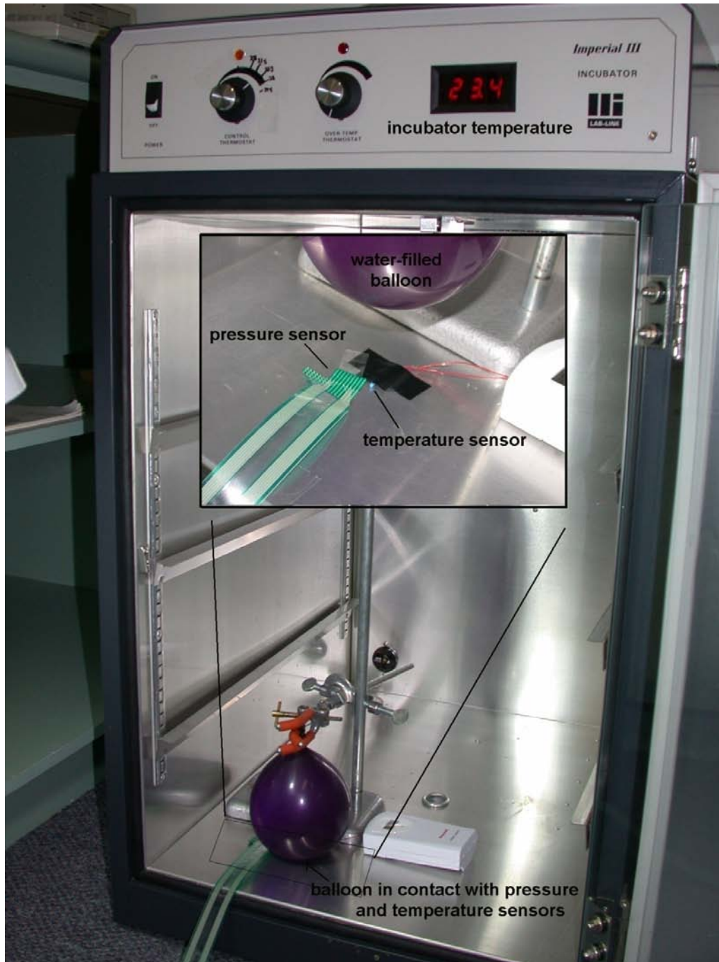
Figure 3-35: Water-filled balloon in incubator in contact with temperature and pressure sensors.
