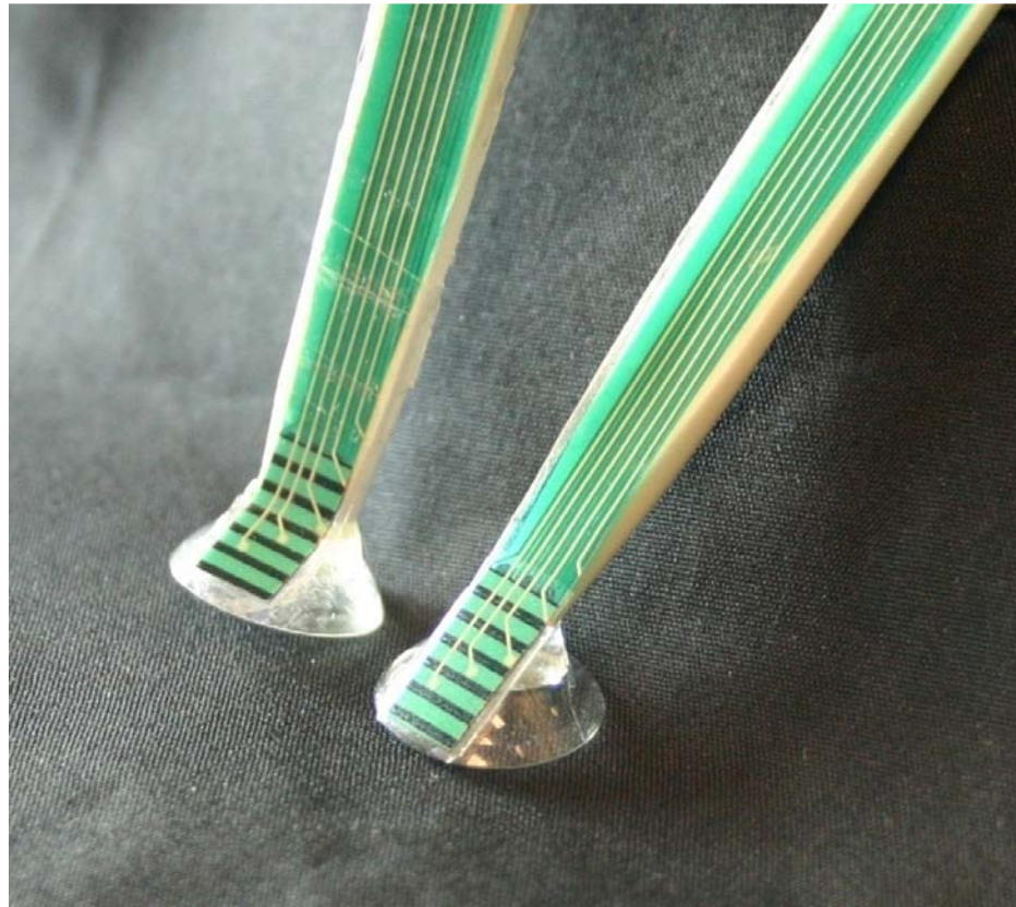
Figure 3-10: The initial bent sensor-contact lens combination (left) which resulted in shearing effects between the layers of the sensor and the flat sensor-contact lens combination (right) with the sensor lying continuously flat from the contact lens surface onto the support beam.
