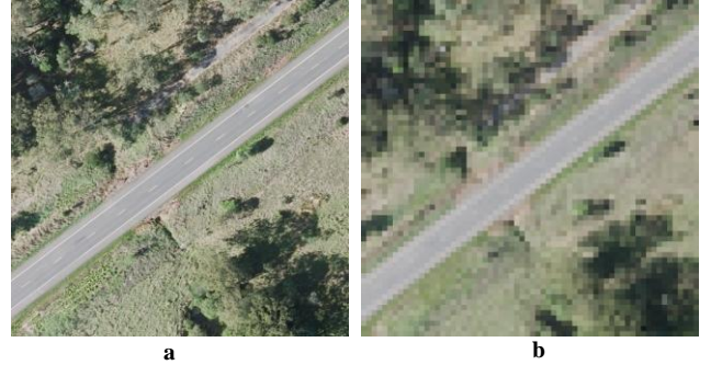
Figure 2. An example of image wavelet decomposition, (a) and (b) are the original and the decomposed aerial images, respectively.
