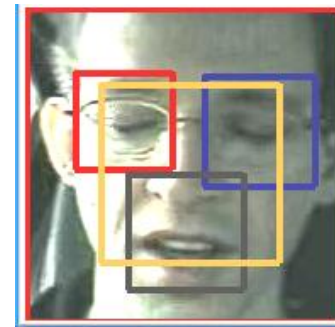
Fig. 9. Diagram of a face and facial feature detection of a AVICAR database image
