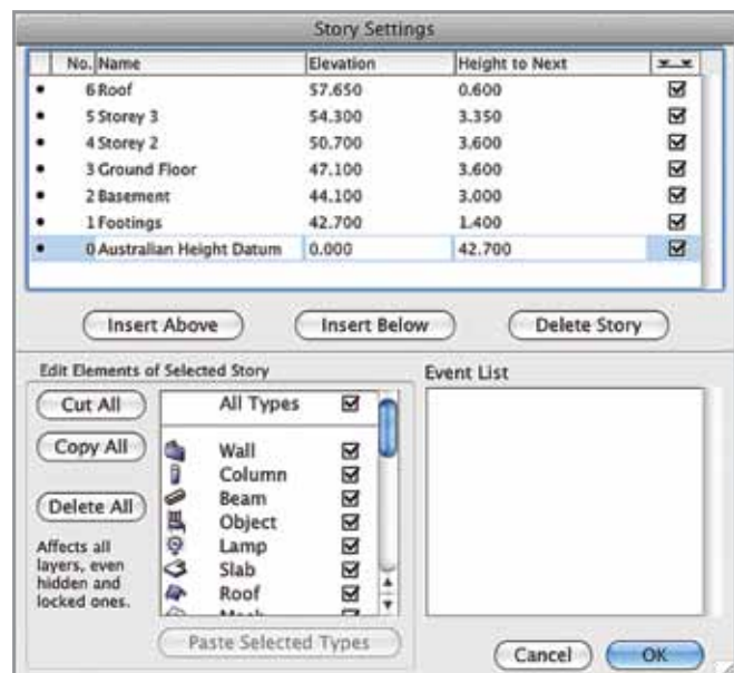
Fig: A1.2 Building Storey Settings
