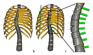
**Fig. 1.** Finite element mesh a. Intact scoliotic spine; b. Surgically altered spinal geometry with the rod and screws shown in green; c. Surgically altered region of the simulated spine, showing the remaining disc annulus elements (yellow) and screws with beam elements (grey wire) simulating the screw heads (screw ends have been lengthened to visualize screw positioning)
