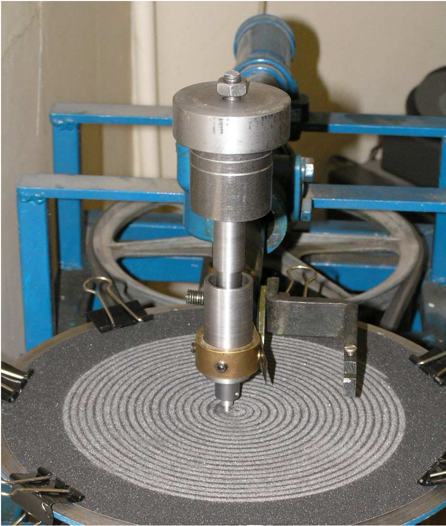
Fig. 1 Experimental pin-on-disk apparatus exhibiting spiral wear track.
