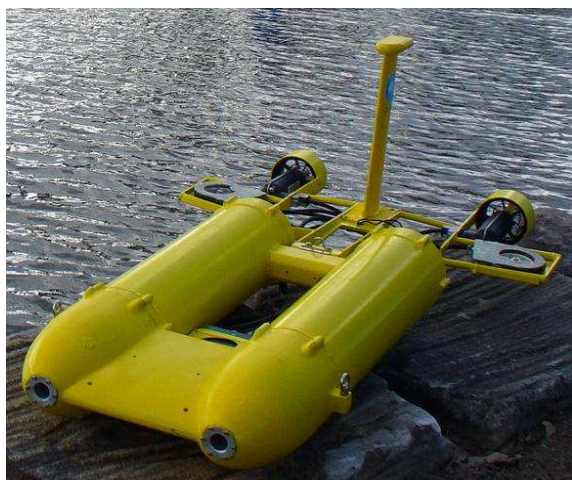
Figure 3: The Starbug MkIII AUV used for experimental studies.
