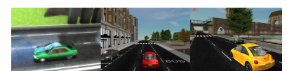
SIVIC (Simulateur Véhicule Infrastructure Conducteur, Vehicle-Infrastructure-Sensor Simulator) is the sensors simulator that we propose to use for development and testing of fusion frameworks and other software. It is developed by the LVIC and increasingly used by transports researchers in France (graphical rendering for machine vision & driving simulation depicted).
