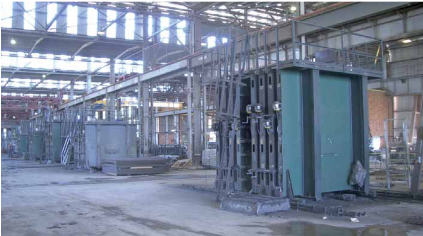
Vertical sound barrier moulds (battery moulds)
