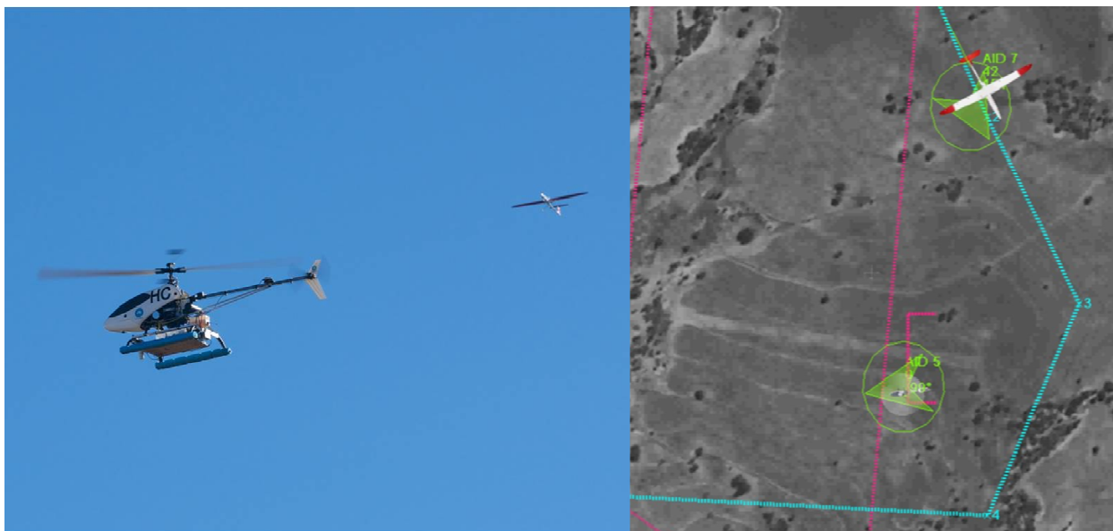
Figure 10. Photo of the two flight test UAS and the situational awareness display showing the CTADS issued by the ADAC (indicated in blue)
