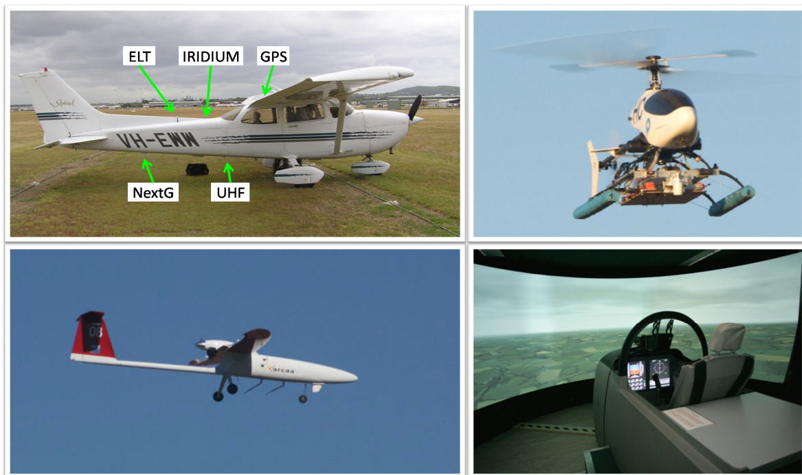
Figure 5. Flight Test Aircraft: ASL, CUAS Heli, Sheffield Piloted 6DOF Simulator, and QUAS Flamingo (clockwise from top left)
