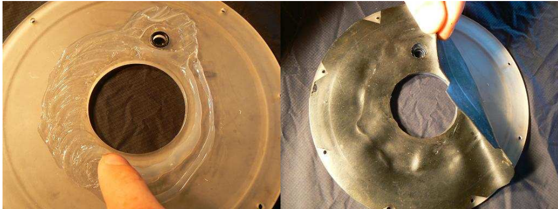
Figure 3-31: Silicon application to the pump mounting plate, (left), the butyl rubber gasket, (right). (Note, the small hole at the top of the mounting plate and gasket allow the LVDT position transducer to protrude through).
