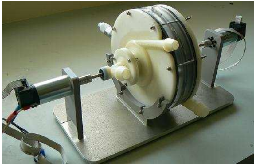
Figure 3-35: Angled view of the prototype housed in the test rig with the twin 20W motors.
