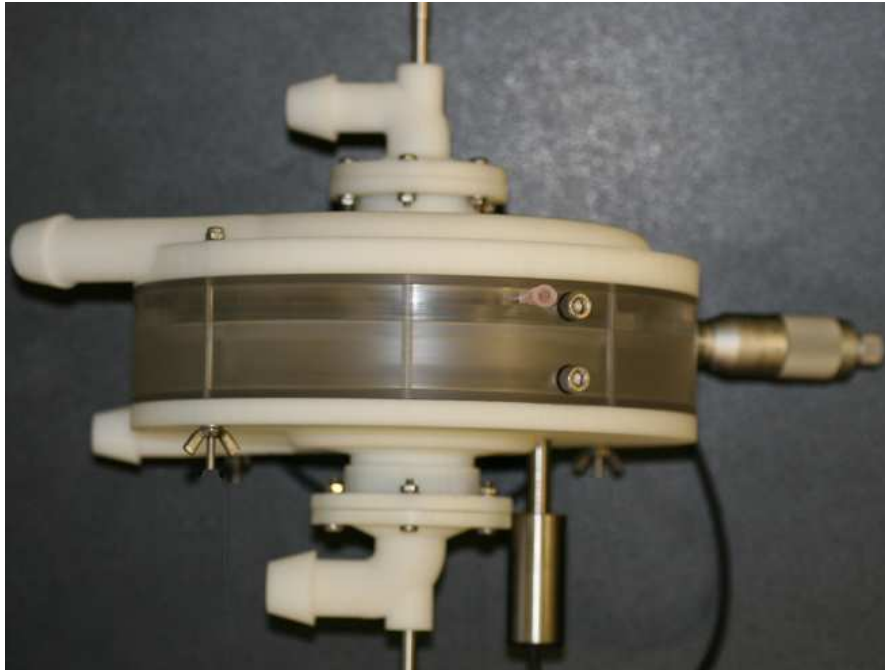
Figure 3-23: Side elevation of Passive Controller BiVAD prototype.
