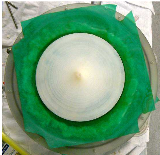
Figure 3-32: Plan view of the Controller body with attached RVAD membrane, (without the butyl rubber gasket). The view is from above the RVAD lower shroud.
