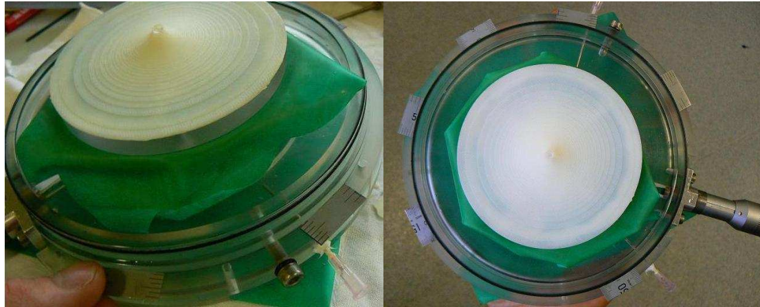
Figure 3-34: Placing the 1.0 mm shims on the Passive Controller Body part 1, (left), plan view of the shims in place before replacing the Passive Controller Body part 2, (right).
