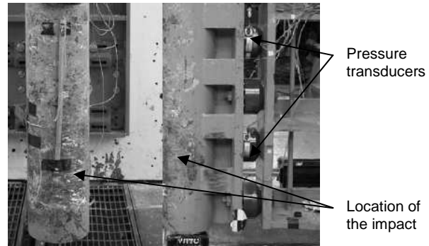
Figure 10: Front and side views of an impacted column
