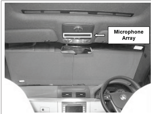
Fig. 1. Location of 8-microphone array used in Australian In-Car Speech Corpus collection.
