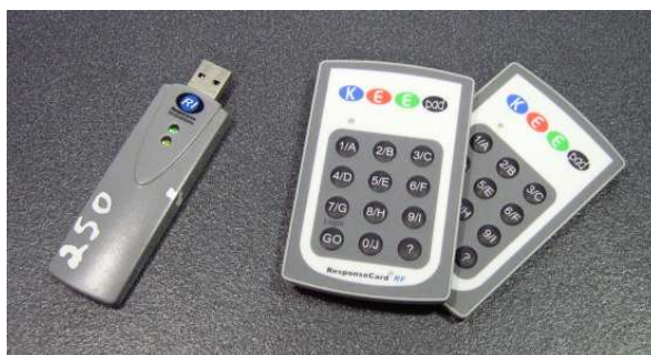
Figure 1: Keypads and the Universal Serial Bus dongle for the “KeePad Interactive” system.
