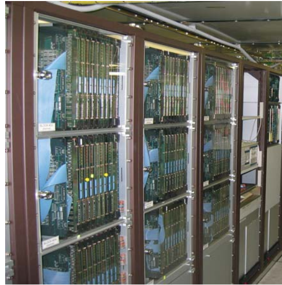
Fig. 2. Hardware correlators at the ATNF, Narrabri, NSW, Australia.
